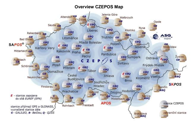
In 2019 the modernization of CZEPOS receivers was completed. CZEPOS services are at present compatible with all accessible satellite systems, i.e. American navigation satellite system NAVSTAR GPS, Russian global navigation satellite system GLONASS, European navigation satellite system Galileo, Chinese BeiDou system as well as with regional Japanese QZSS.
